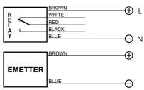
**Note:** in case of inductive loads it is necessary to connect one diode in antiparallel at the edges of the load.
